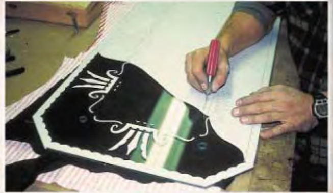
Custom glass fixtures require great attention to detail. Here, crown and scallop designs are carefully cut into a mask before sandblasting to recreate an Art-Deco lens.
